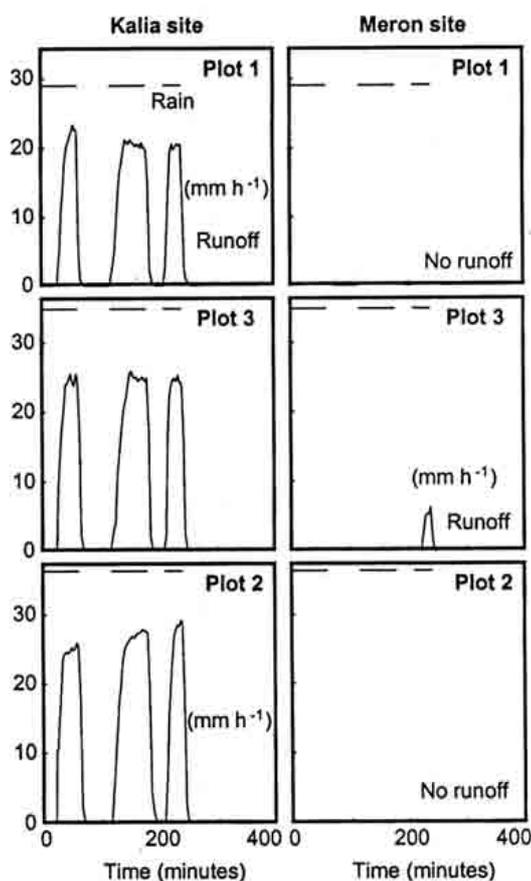
Figure 4. The overland flow response to the simulated rainfall at the driest site, Kalia, compared with that of the wettest site, Meron.
