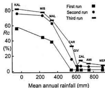
Figure 8. Overland flow coefficients ( $R_c$ , %) at different climatic conditions. The values are averages for the three plots.
