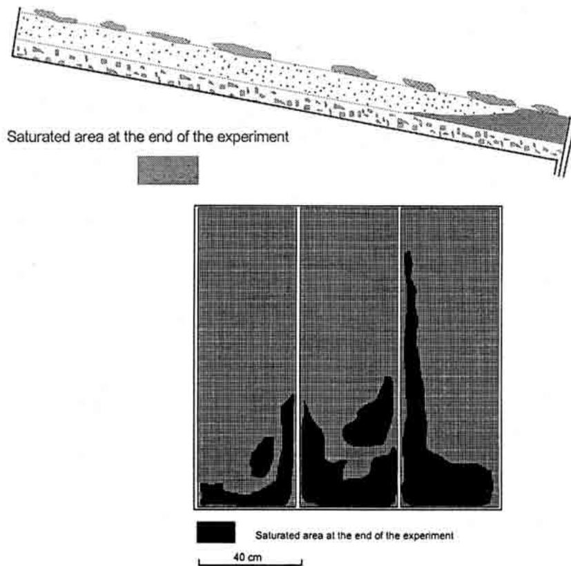
Figure 7. An example from site Amirim of the saturated area after the experiment: a. A cross section; b. Overview.
