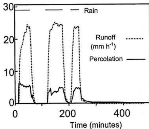
Figure 3. Typical results of the experiments for Kalia. The first run, on relatively dry soil lasted for 60 minutes. The second run began after 60 minutes break and lasted for 60 minutes. The third run, after a break of 30 minutes lasted for 30 minutes. Overland flow and percolation were measured at three minutes intervals.
