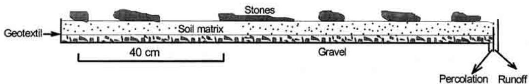
Figure 2c. The soil stratification within the plots. 4 cm of soil covered by rock fragments similar to the natural conditions is lying over a geotextile sheet and 2 cm of gravel.
