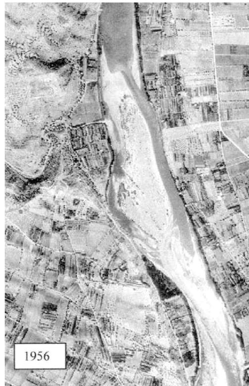
Figure 7. Vegetation encroachment downstream in the Ebro River due to the lack of floods (Vericat & Batalla, 2003).
