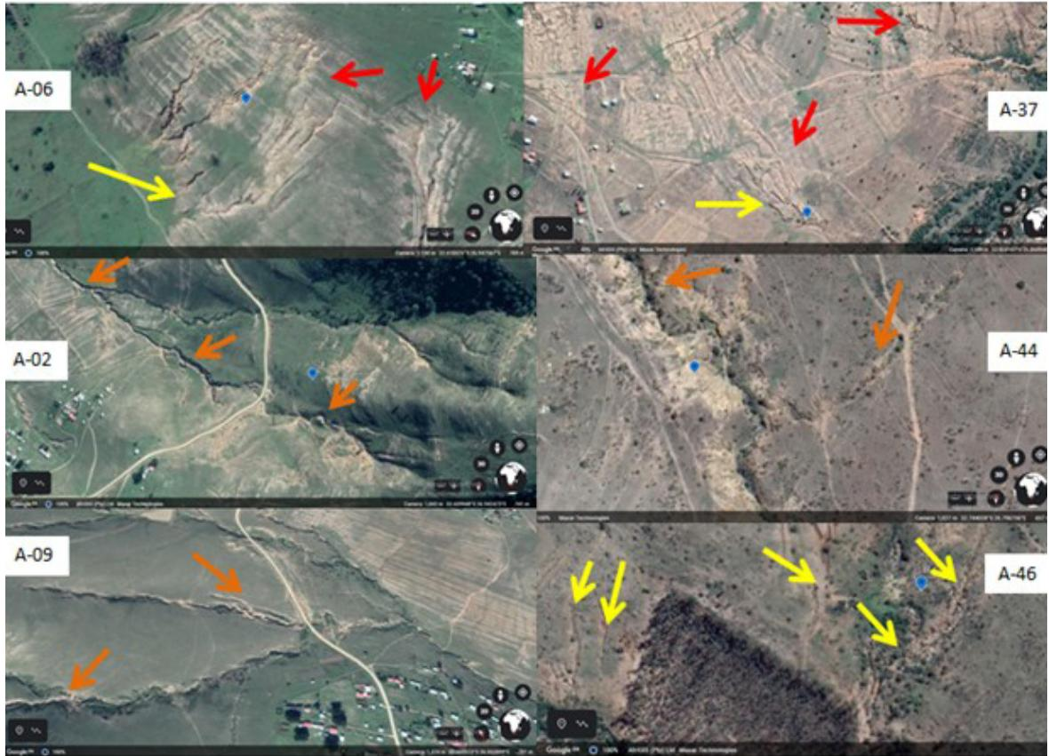
Figure 5B. View of tracks of soil erosion by water (Areas of mass waste resulting from rill erosion are shown with red arrows, rill erosion tracks are shown with yellow/orange arrows)
