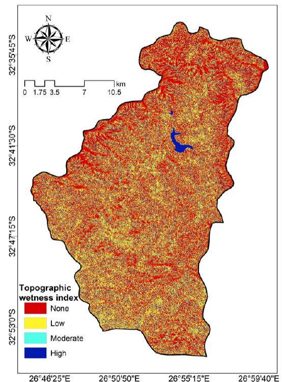
Figure 3B. Topographic wetness index of Tyume Basin.
