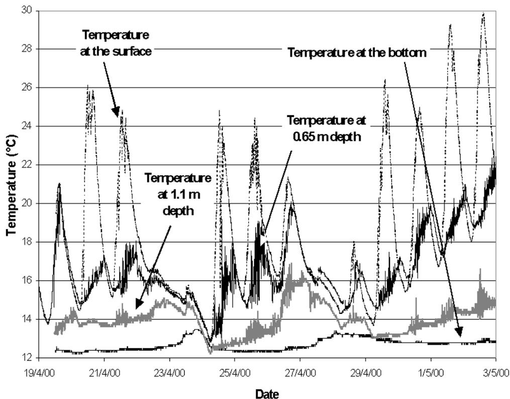
**Figure 6** Pond water temperature profiles
