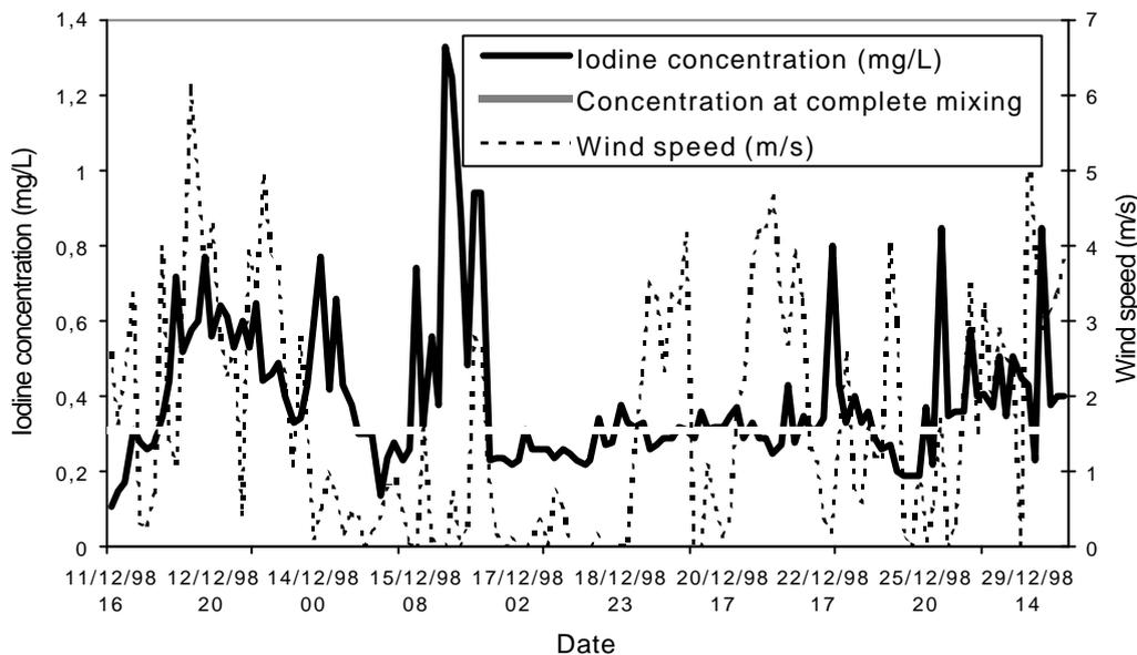
**Figure 2** Winter test - tracer concentration at the outlet of the pond and wind speed (the tracer was injected at 10 a.m. on Dec 11)
