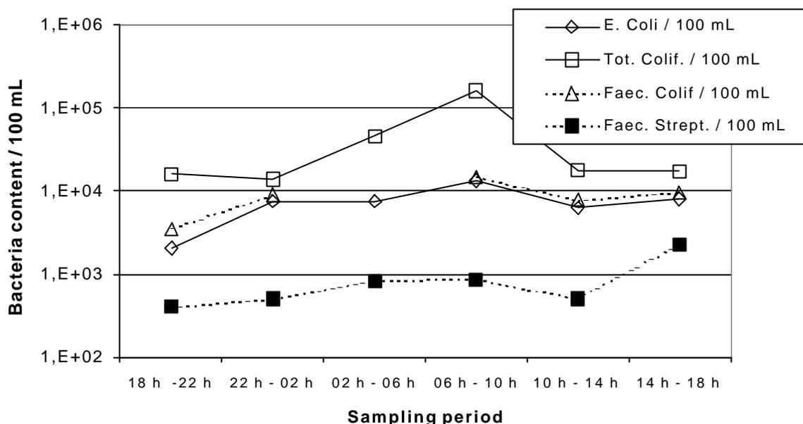
**Figure 7** Round the clock monitoring of bacteria content at the pond outlet
