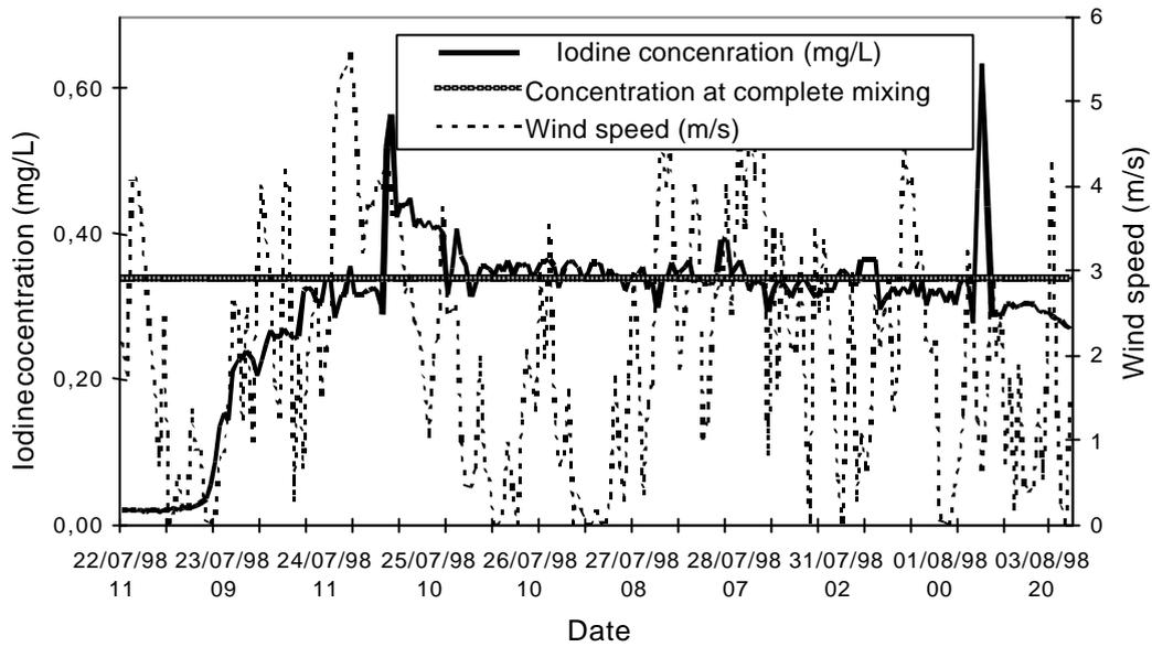
**Figure 4** Summer test – tracer concentration at the outlet and wind speed
