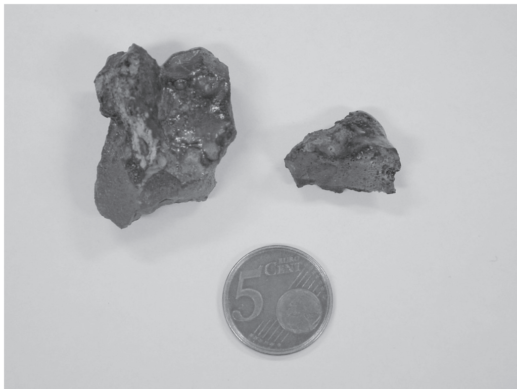
3 Vacuolar slag found in Zamora which was confused with a meteoritic fragment
